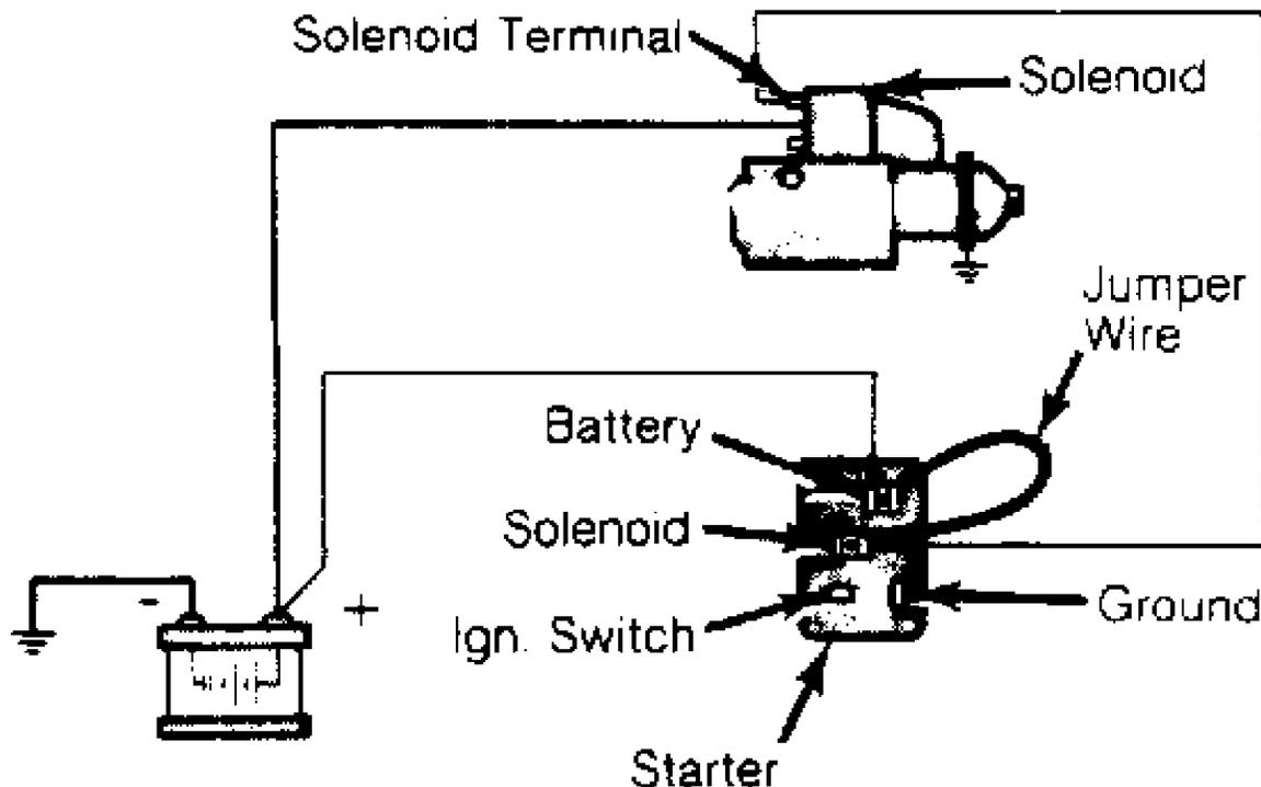
Fig. 1: Typical Starter Solenoid Test
