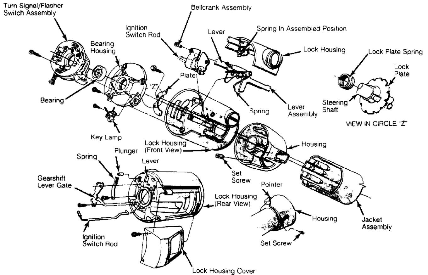
Fig. 5: Exploded View of Column Shift Steering Column Housing
