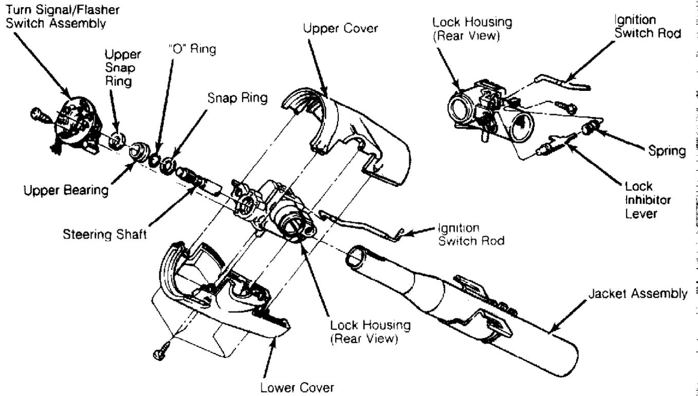
Fig. 6: Exploded View of Floor Shift Steering Column Assembly
