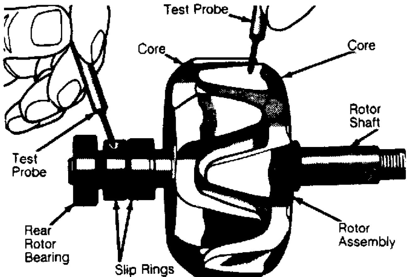
Fig. 12: Testing Rotor Coil for Ground
