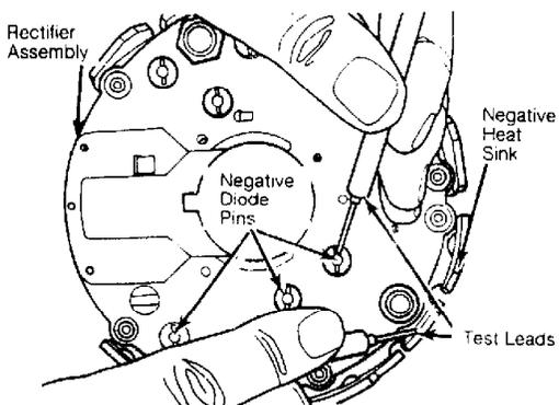
Fig. 17: Testing Negative Diodes
