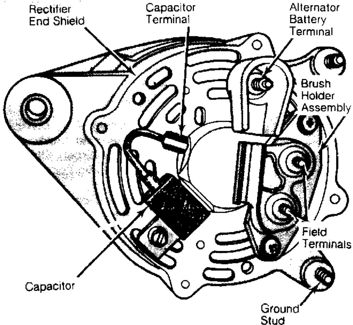
Fig. 1: Rear View of Bosch 40/90 Alternator
