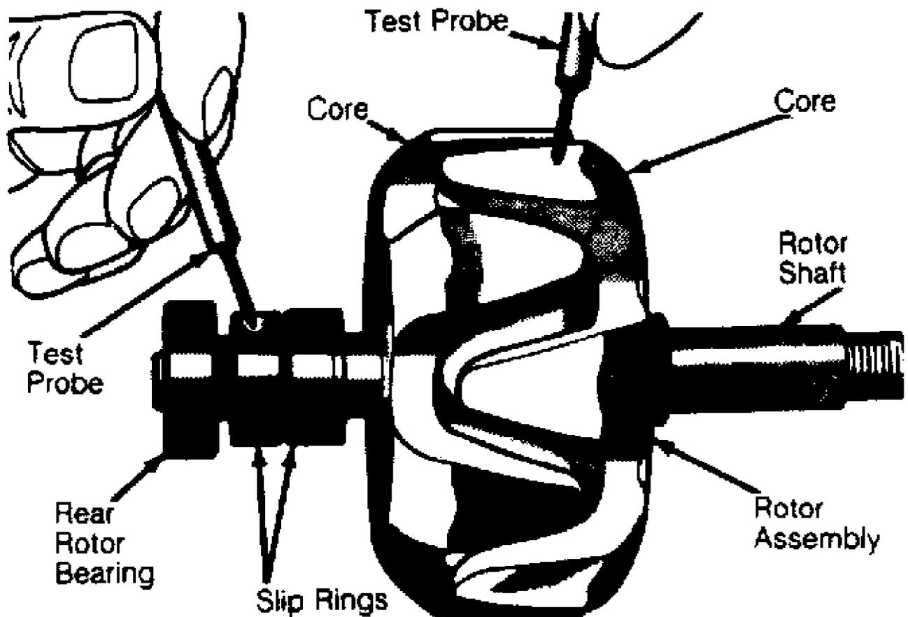
Fig. 12: Testing Rotor Coil for Ground
