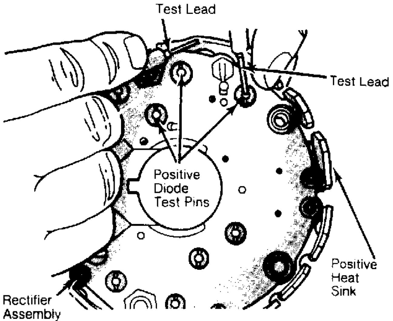
Fig. 16: Testing Positive Diodes
