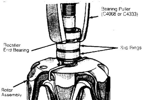
Fig. 10: Removing Rectifier End Bearing
