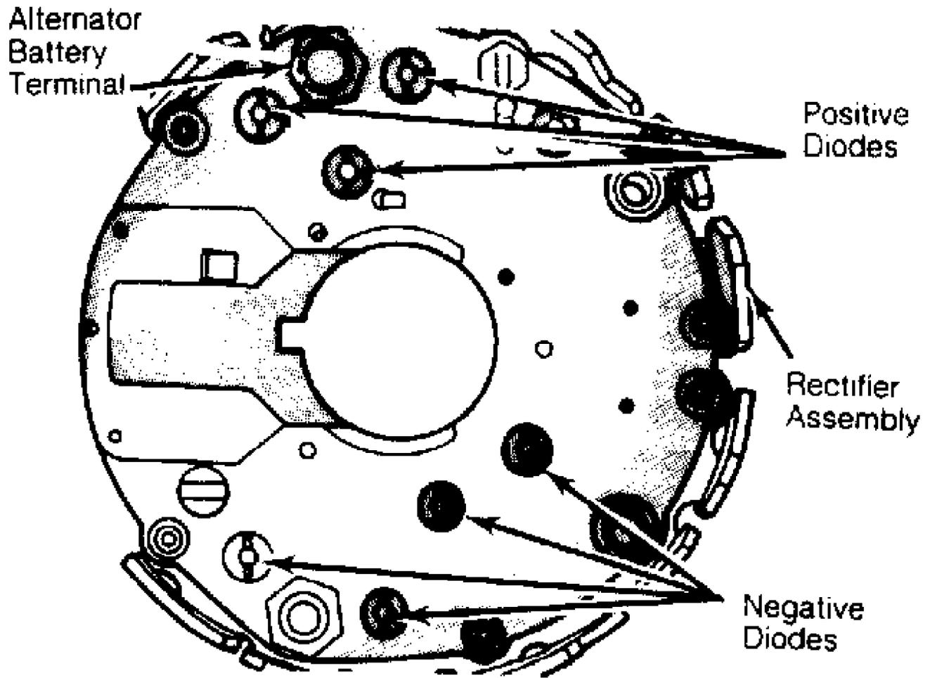
Fig. 15: Checking Rectifier Assembly
