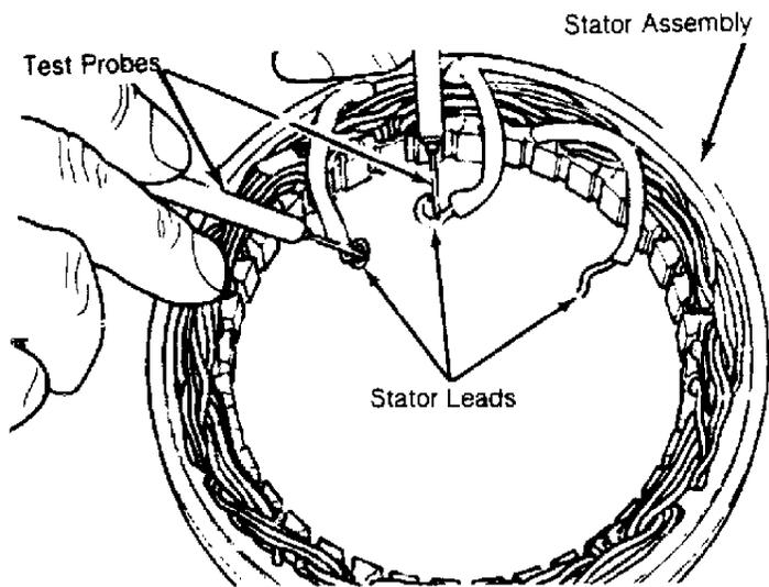
Fig. 14: Testing Stator Coil for Open or Ground
