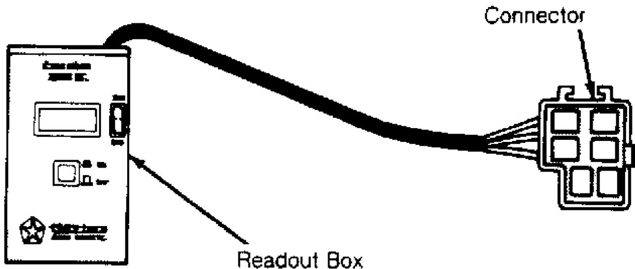
Fig. 2: View of Diagnostic Readout Box
